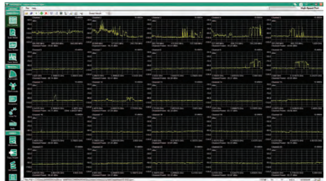
Use the High Speed Port Scanner Monitor Multiple RF Channels with a Single Field Master MS2090A on a Single PC Monitor
