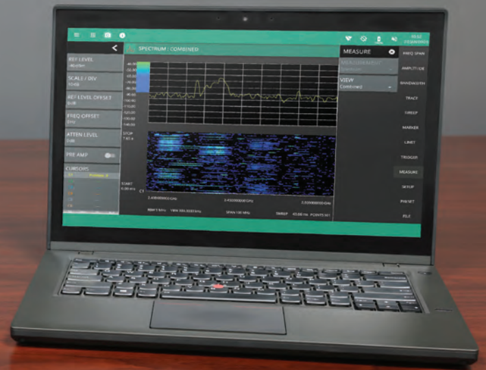
Laptop PC Running Remote GUI Application with Wi-Fi Connection to the Field Master MS2080A
