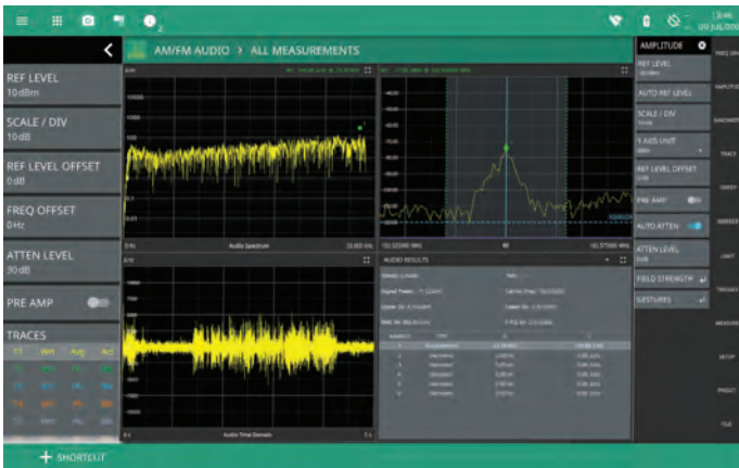
AM/FM Modulation Measurement Option Delivers the Most Comprehensive Measurement Suite in a Remote Spectrum Analyzer. The RF Spectrum, Audio Frequency Spectrum, Demodulated Audio in the Time Domain (oscilloscope format), and Numeric Results for Key Parameters are all Displayed on the Remote Software Screen
