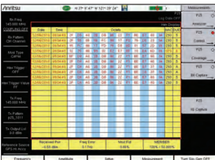
The P25 Control Channel Display Provides a Hex Display of the Trunked Downlink Data in Hex Format. Anritsu Offers a Free Software Script to Convert the Hex Information to Text Messages.
