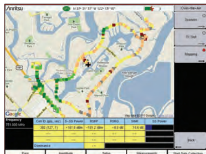
Over-the-Air Measurements – Tx Test By Looking at the Reference Signals of MIMO Antennas One can Determine if MIMO is Working Properly. If the Delta Power is too Large, There is an Issue.
