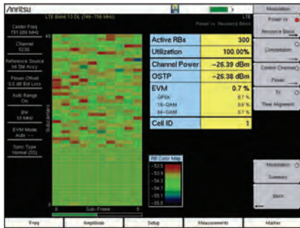
Modulation Quality – Power vs Resource Block A High Utilization of the Resource Blocks Would Indicate a Cell Site in Nearing Overload and it May be Appropriate to Start Planning for Additional Capacity
