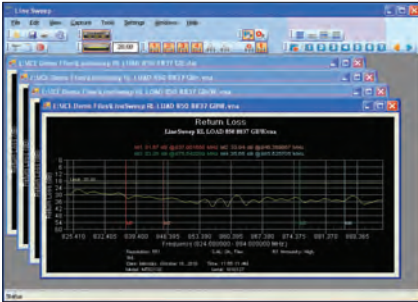
Trace Validation Marker and Limit Line Presets Allow Quick Checks of Traces for Limit Violations
