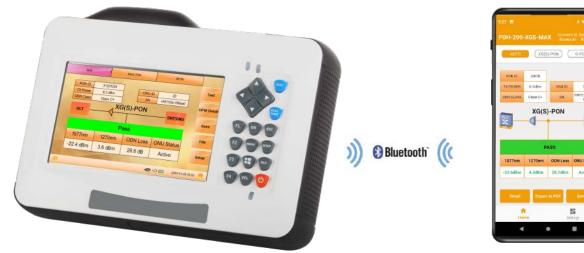
With the upgrade of GPON networks to XG(S)-PON, we have launched the new FOH-200XGS-MAX to apply for the installation and maintenance testing of the upgraded Combo PON network. By connecting FOH-200XGS-MAX in series to the PON network, we can quickly and accurately extract OLT and ONU information, suitable to test GPON and XG(S)-PON at the same time.
