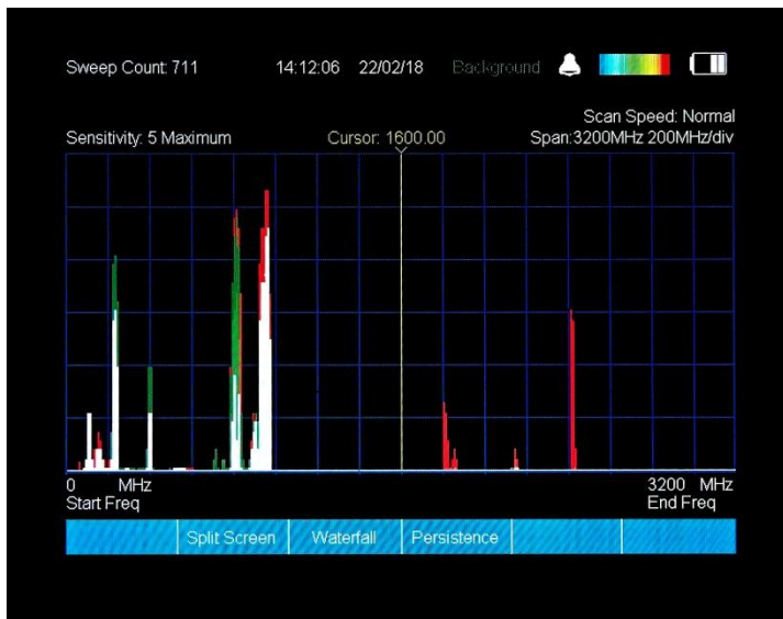
Main Screen - Live signals (white), Historical signals (red) and Background recorded signals (green).
