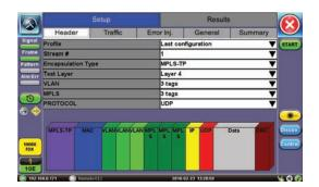
TCP Throughput Compliant with RFC 6349 Stateful TCP Test at line rate TCP Client and Server modes Compatible with iPerf Client/Server MTU search per RFC4821 Round Trip Time Measurement Configurable TCP Window sizes Multi-Window size tests
