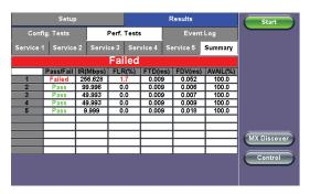
Simple summary Pass/Fail results tables and drill down capability with detailed measurements (Frame Loss, Frame Transfer Delay, Frame Delay Variation, Availability) for each service.
