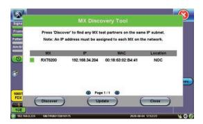
Discovery function to all VeEX devices within subnet or manual control of VeEX test sets in routed network
