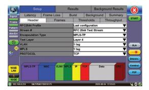
Automated tests compliant with RFC2544 with configurable threshold values and maximum transmit bandwidth settings Throughput, Latency, Frame Loss, and Back-to-Back (burst) tests Frame sizes: 64, 128, 256, 512, 1024, 1280, 1518 bytes and 2 user configurable frames
